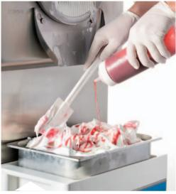
To better variegate gelato in the tray, the beater speed can be reduced, even stopping extraction completely allowing the easy distribution of toppings. Then, increasing beater speed again, extraction continues. The shelf mat is designed to firmly hold trays and tubs in position while gelato is being worked on.
