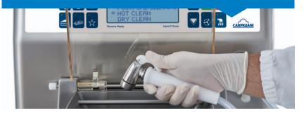
Even the cleaning of the surfaces is quick because the Scoth-Brite treatment of the stainless steel makes it resistant to stains and fat residues.
